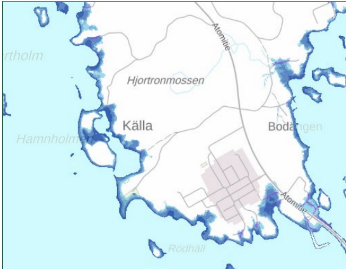
Figure 4-1. Flood map of the Källa planning area. The possibility of a very rare sea flood is likely to occur once in about 1000 years (1/1000 years). Therefore, it is extremely unlikely (0.1 %).
