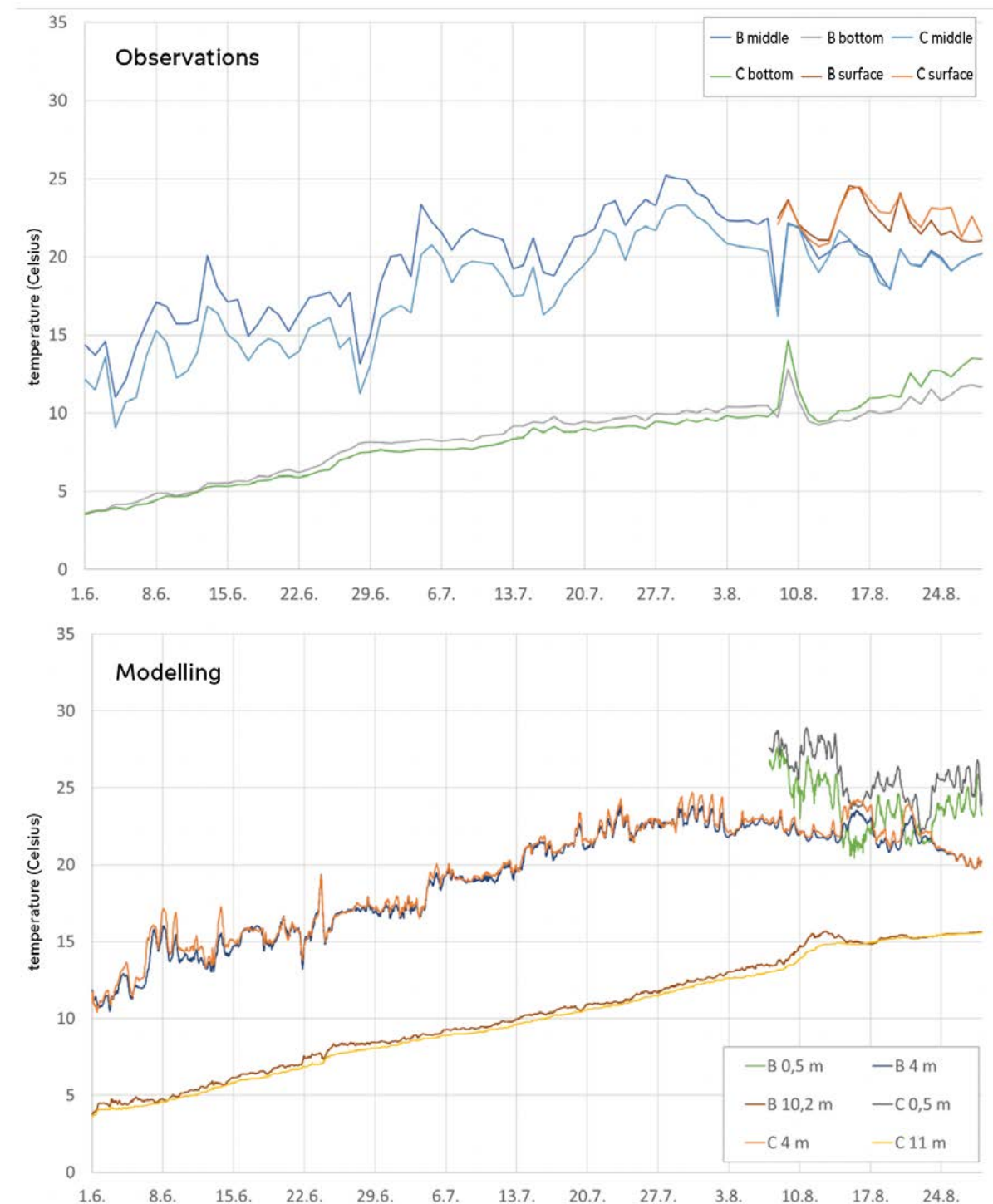
Figure 4-8. Hästholmsfjärden, buoys B and C, the observed (above) and modelled (below) water temperature at various depths in June – August 2011. The fluctuation in the observations at the beginning of August is due to the maintenance of the measuring transducer.
